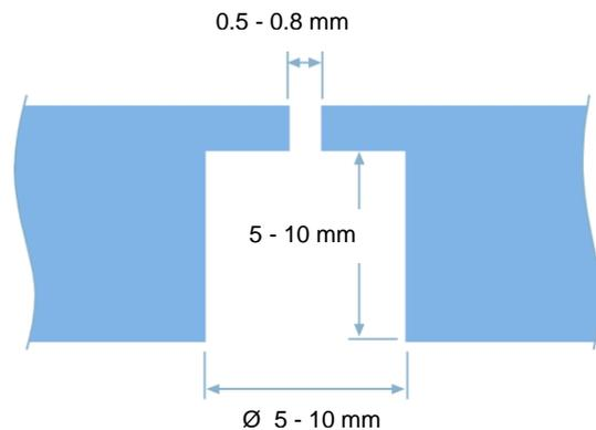
Fig. 3: Sketch of vents during thermoforming
